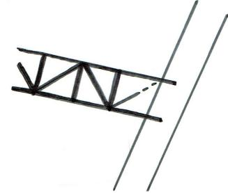
4. CONNECTION STEEL - CONCRETE EACH BRIDGE HAS 4 ANCHORED CONNECTIONS IN REINFORCED CONCRETE CORE WALL.
